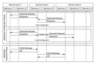
Fig. 5. Application Configuration and Execution Phase.
