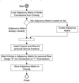
Fig. 6. Algorithm for Documentation of Connection Establishments.
