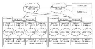
Fig. 8. Prototype Setup.
