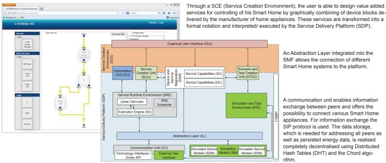
An Abstraction Layer integrated into the SMF allows the connection of different Smart Home systems to the platform.
