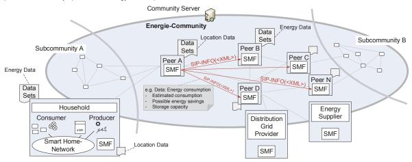
The concept provides a mechanism for convenient networking of households, energy suppliers, distribution network operators and others with the objectives cost savings, avoidance of grid expansion, energy savings, CO<sub>2</sub> reduction etc.
