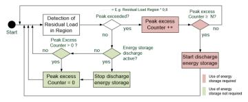
Fig. 5. Algorithm for peak load reduction
